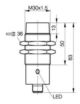
Inductive Sensors BES 516-548-S 4-H M30x1.5 x 83 normally-open Sn=15mm unshielded
